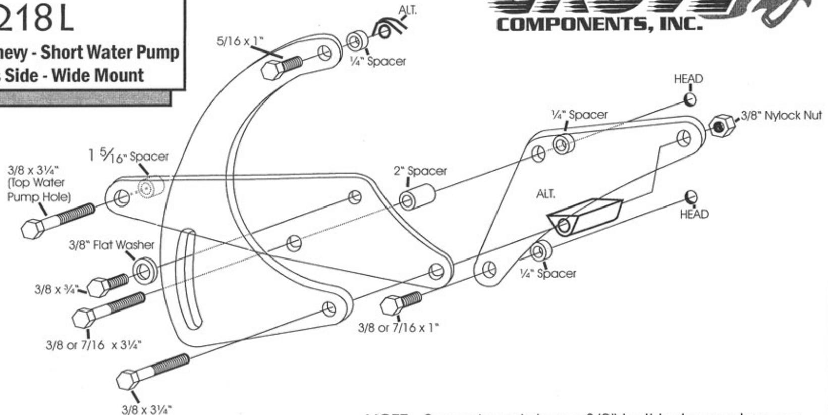
(We use a belt length of 58-59" with this mount on installations in our shop. However; this can vary with the diameter of your pulleys.)
